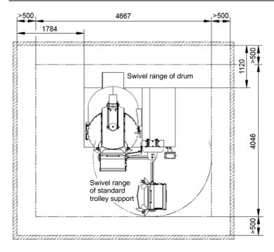
The work area around the machine is at least  $0.5\,\mathrm{m}$  on all sides; for maintenance work it is at least  $1\,\mathrm{m}$ ; if used as passage way, it is at least  $1.2\,\mathrm{m}$ .
